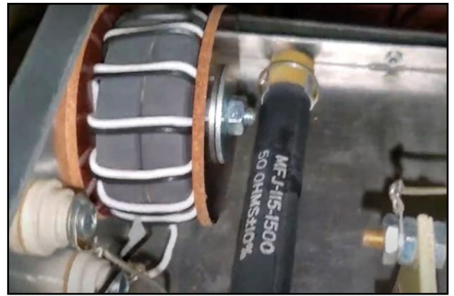
Fig. 5 – A built-in balun in an MFJ tuner.
