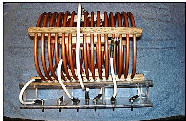
Fig. 4 – Tapped inductors have wires attached at various points. By selecting a particular wire, you get a fixed amount of inductance.
