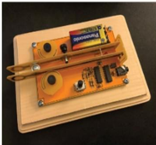
The Cric-Key kit from Four State QRP group comes together in about 2 hours to give you a paddle and keyer all in one.
