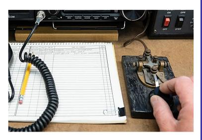
• At the receiving end, the listener could use filtering techniques to block everything except the frequency the CW operator was using. This greatly reduced the effects of noise and interference. The signal could then be amplified and made louder, which made the CW signal much easier to understand.
