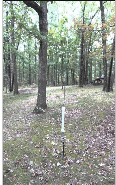
**In addition to the club's two OCFD Windom antennas, two verticals were used, one of which was K5NZV's nifty homemade coil vertical show above**
