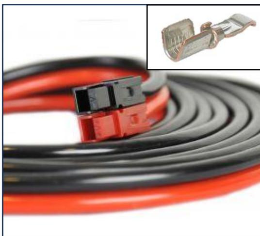
PowerPole connectors shown with red/black cable. Figure 5 shows 10-gauge wire being used, which would require the 45-amp connector mentioned earlier.
