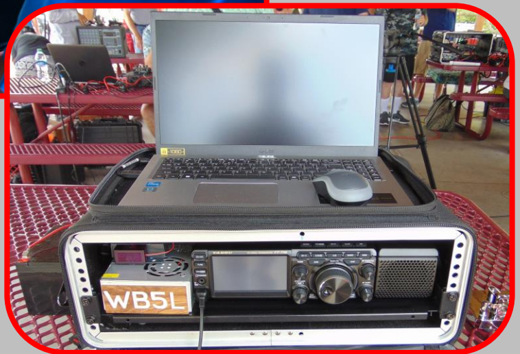
The super RIB (Rig In a Box) furnished by Glenn-WB5L, one of the rigs used for Digital station
