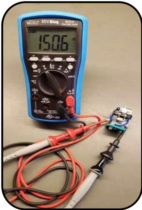
Figure 2 – Measuring the relay coil resistance with an Ohmmeter. The energizing current can be calculated with Ohm's law: ( I = V/R ).
