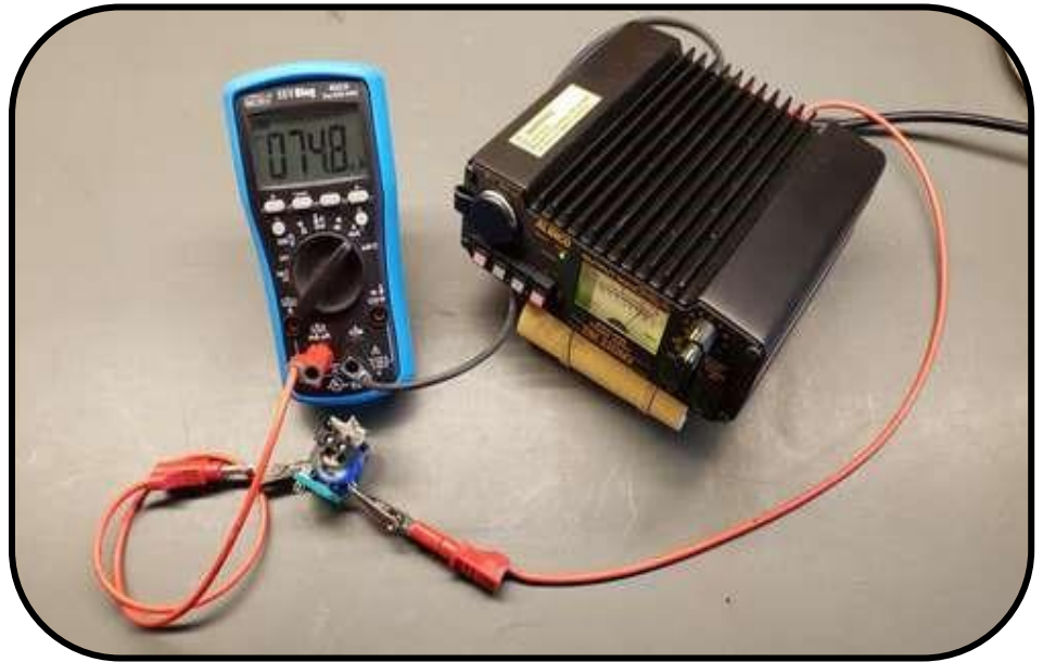
Figure 3. Measuring the relay energizing current with an ammeter. This setup is using the same power supply as the transmitter (i.e. 13.8V), but the current should be measure with the actual power supply that you intend to use for the relay. The setup will energize the relay coil so you can see if the contacts are working.
