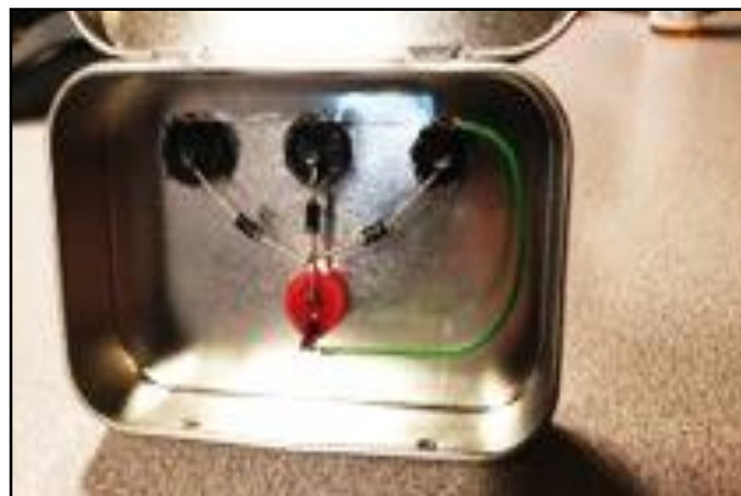
Figure 7. Internal wiring for a keying line interface. Note the striped ends of the diodes are connected to the transmitter keying line connector. Additional connectors and diodes could be added to control additional devices from the keying line..
