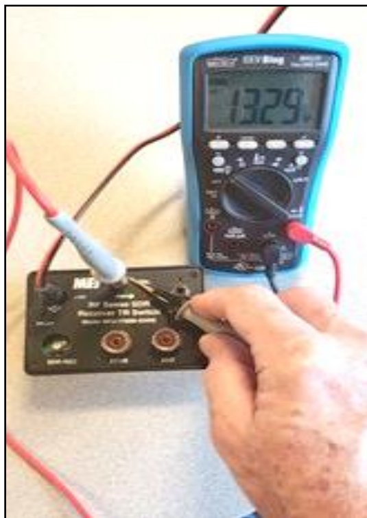
Figure 3. Measure the control voltage with a multimeter in voltage mode. In this case, the control voltage is +13.29V. Also, check that the voltage polarity matches your transmitter specifications.
