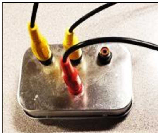
Figure 6. Keying line interface for multiple devices in an Altoids tin. The red lead connects to the transmitter keying line, and the yellow leads connect to the controlled devices.
