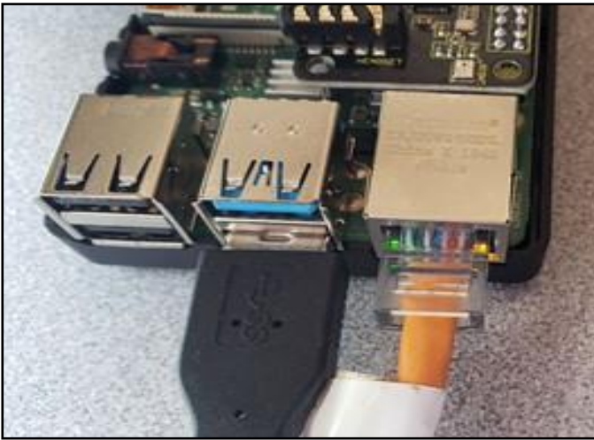
Figure 3. The hardwired ethernet connection using a RJ45 modular connector.
