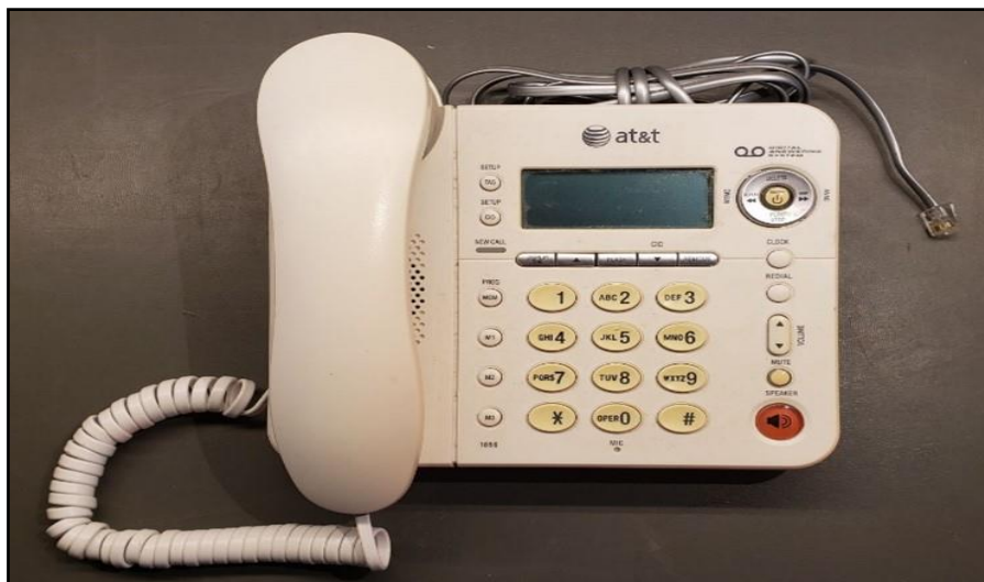
Figure 2. Land line telephone using RJ22 connectors on the coil spring handset cord and RJ11 connectors for connection to the telco wall socket.
