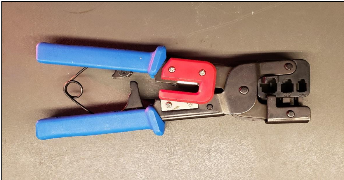
Figure 7. A ratcheting type of crimper provides a consistent quality crimp on RJ modular connectors.
