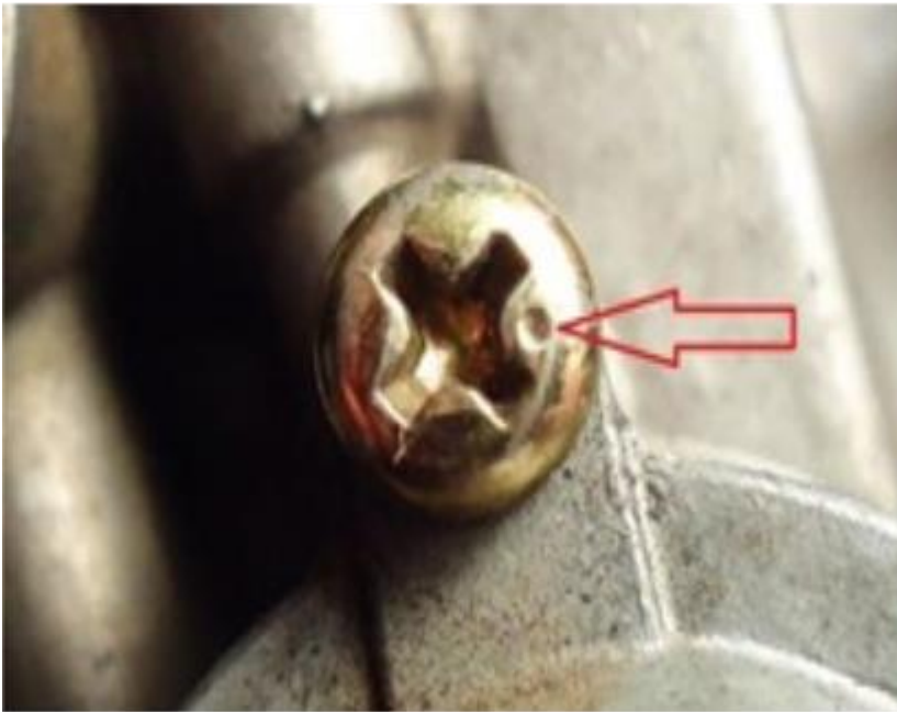
Figure 3. The dot on a screw head indicates a JIS screw, and some JIS screws are marked with a small “X” as seen in figure 1. Just to make life more interesting, not all JIS screws have the dot or the “X”.
