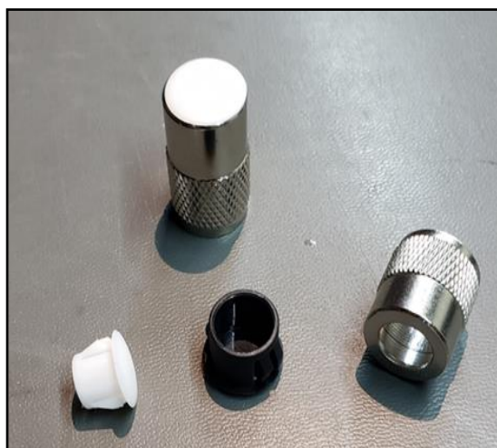
Figure 2 – The backside of the PL-259 nut sealed with commercially available plugs (i.e. Home Depot / Lowes)
