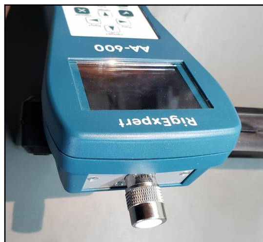
Figure 3 – Antenna Analyzer connector protector
