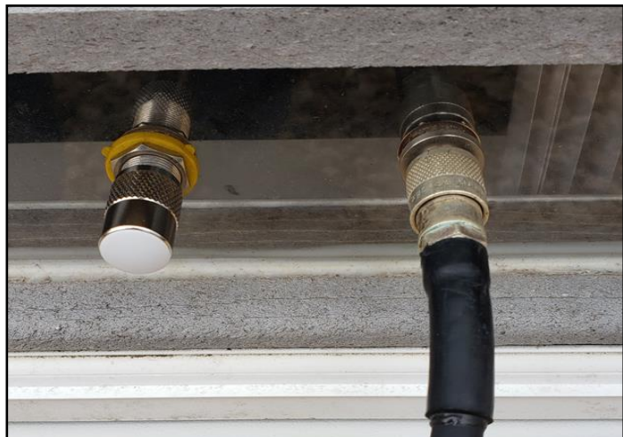
Figure 4 – Antenna Analyzer connector protector
