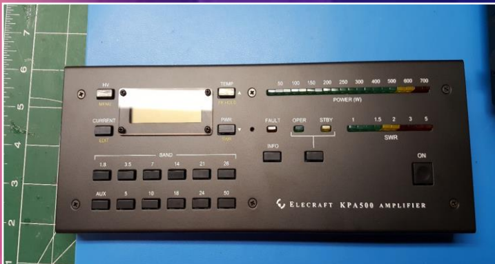
Front panel showing the LEDs and buttons through the front panel to operate the KPA-500
