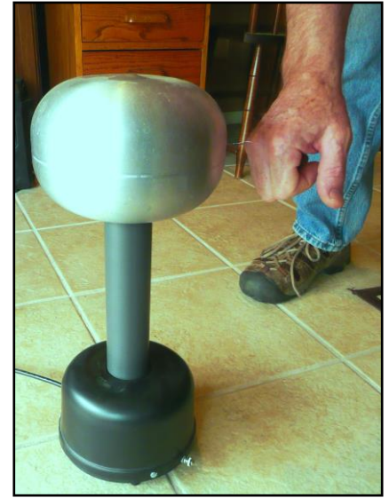
The van de Graff throwing a very small bolt to the knuckle. Unmolested, it will arc to the floor.
